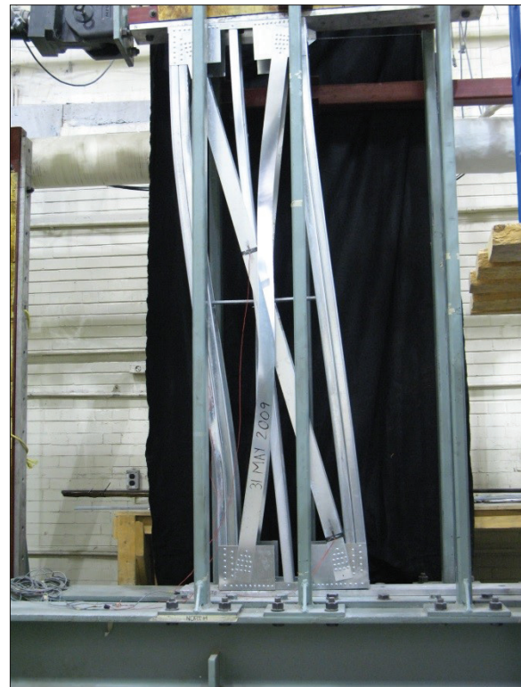
Figure 4-6. Narrow strap-braced wall.
