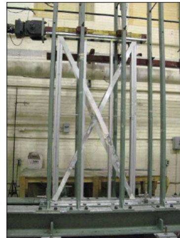
(c) Typical strap-braced wall specimen in test rig (adapted from Comeau 2008 Figure 2.21)
