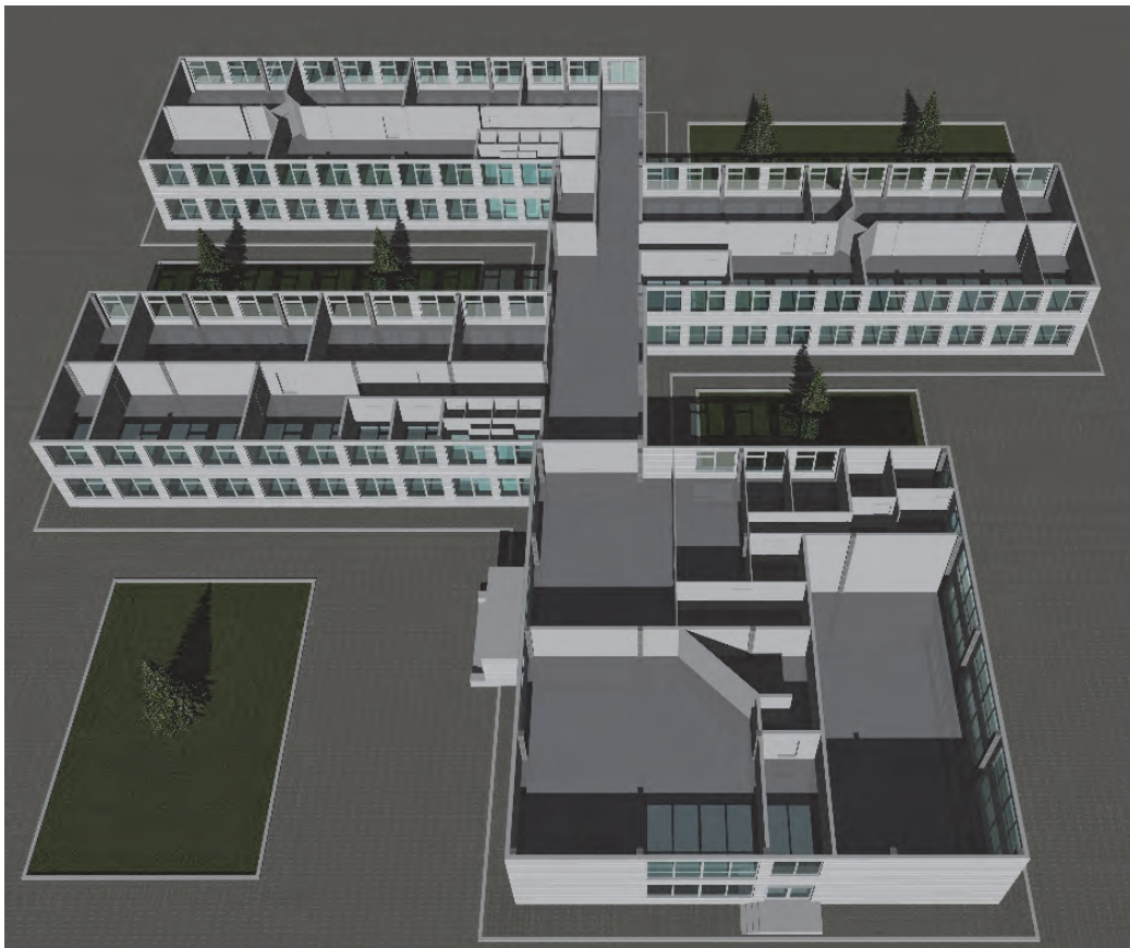
Figure 4-10 Typical wall layout for two-story Typology D-1 school buildings (EEC et al., 2015).
