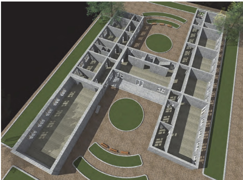
Figure 4-6 Typical wall layout for two-story Typology A school buildings (EEC et al., 2015).
