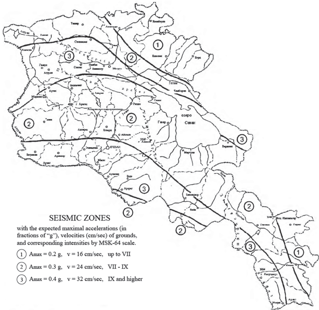
Figure 3-1 Seismic hazard map from the Armenian Building Code (Ministry of Urban Development, 2006).
